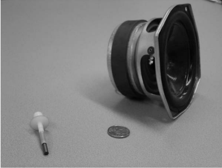
Figure 4.6 Left: Magnet system of the prototype (MM3c shown in Fig. 4.7) of the optimal low- Bl driver (only 3 g and 4.5-mm diameter) with a 50 Euro cent coin. Right: a small woofer of 13-cm diameter and about 1 kg
