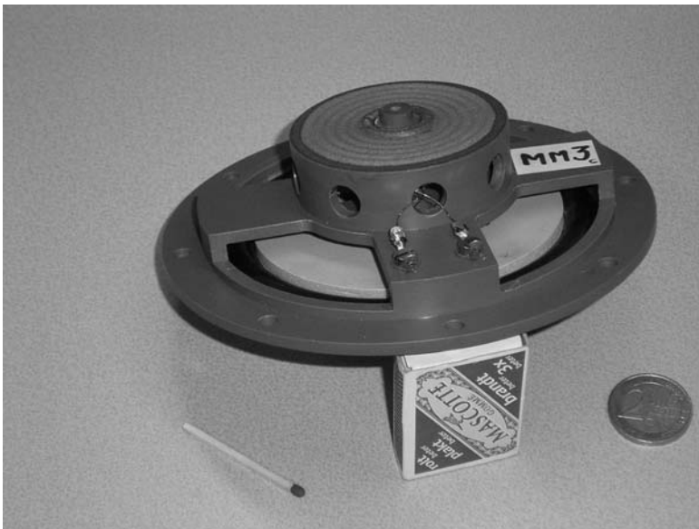
Figure 4.7 Picture of the prototype driver (MM3c) with a 2 Euro coin and ordinary matches. At the position where a normal loudspeaker has its heavy and expensive magnet, the prototype driver has an almost empty cavity; only a small moving magnet is necessary, which is visible at Fig. 4.6 (left side)
